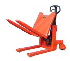
The pallet tilter lifts, tilts and transports crates or boxes on pallets.
